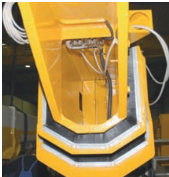
The cabling is securely housed in the telescopic arms between the work platform and the chassis
