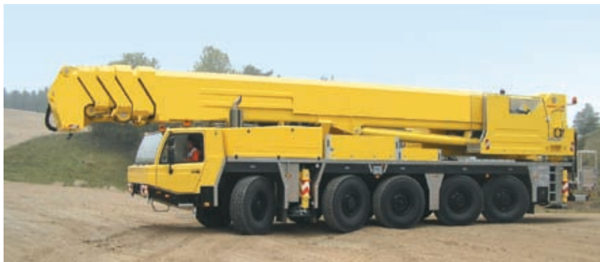
60 tons power: The Faun crane chassis with Wumag aerial work platforms can even be transported without special approval in road traffic
