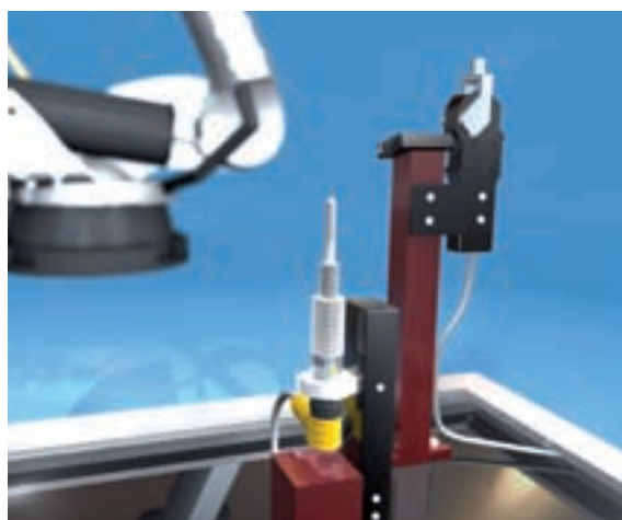
The magnetic field sensor forms the heart of the “smart location bolt”
