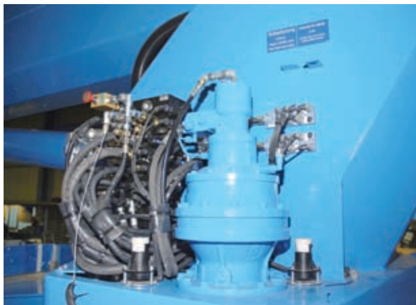
Emergency operation on the device control block: The actuator sensor boxes withstand wind and weather as well as temperatures between -20 and +80 °C
