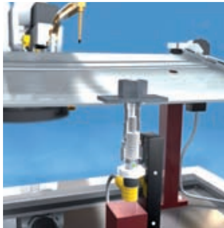
After the operator has placed a welding nut on the location bolt, the sensor sends a signal to the PLC
