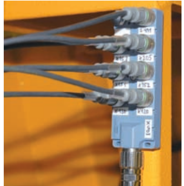
Tight: The actuator sensor box with M12-Push-Pull plug-in connectors meets IP69K degree of protection
