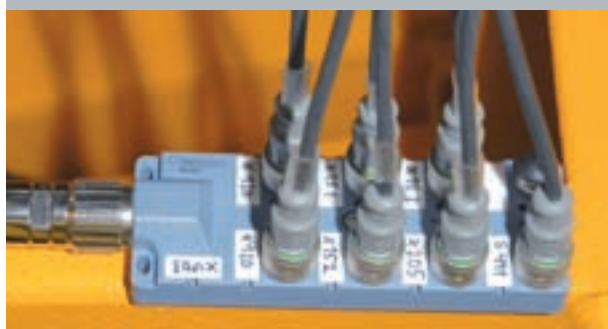
Turck boxes with rapid plug-in systems on Wumag's aerial work platforms are extremely leakproof Page 32
